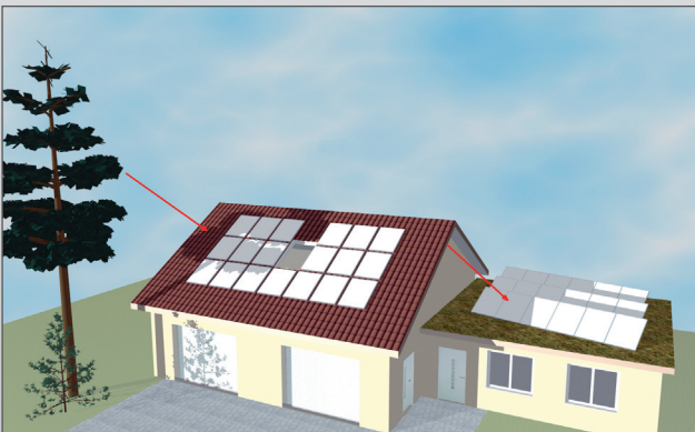
Structural shading objects can be displayed in the 3D-module to allow analysis during project planning.
